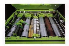
The modern high speed universal tubing machine is arriged for the manufacture of flush-out and stepped-end tubes, with oxithout gussets. The large format area ensures a wide usage possibility.
